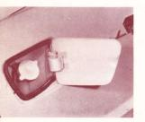
The gas filler opening is covered by a hinged door with a strong over-center-design spring which positively holds the cover open or closed.
