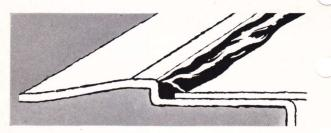
A new sealing technique is an outstanding feature of the 1955 body. At points where body panels are welded together, a groove is formed at the overlapping edges of the panels and filled with mastic material before assembly. This provides a tight seal after welding and keeps out water and dirt. The technique is particularly valuable in the floor panels, which are splashed by mud and moisture from the road.
