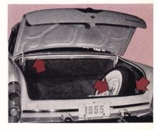
The Dodge luggage compartment lid may be locked or merely latched as you prefer. Turning the key locks the lid securely. But if it happens to be more convenient to leave the compartment unlocked, the latch holds the lid firmly closed. It then can be reopened easily by simply pushing the button—a convenience on shopping trips, picnics and similar situations.
